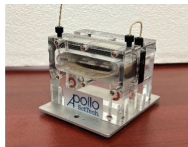
Figure 3. Water-jacketed flow cell (Inside Cary60)
