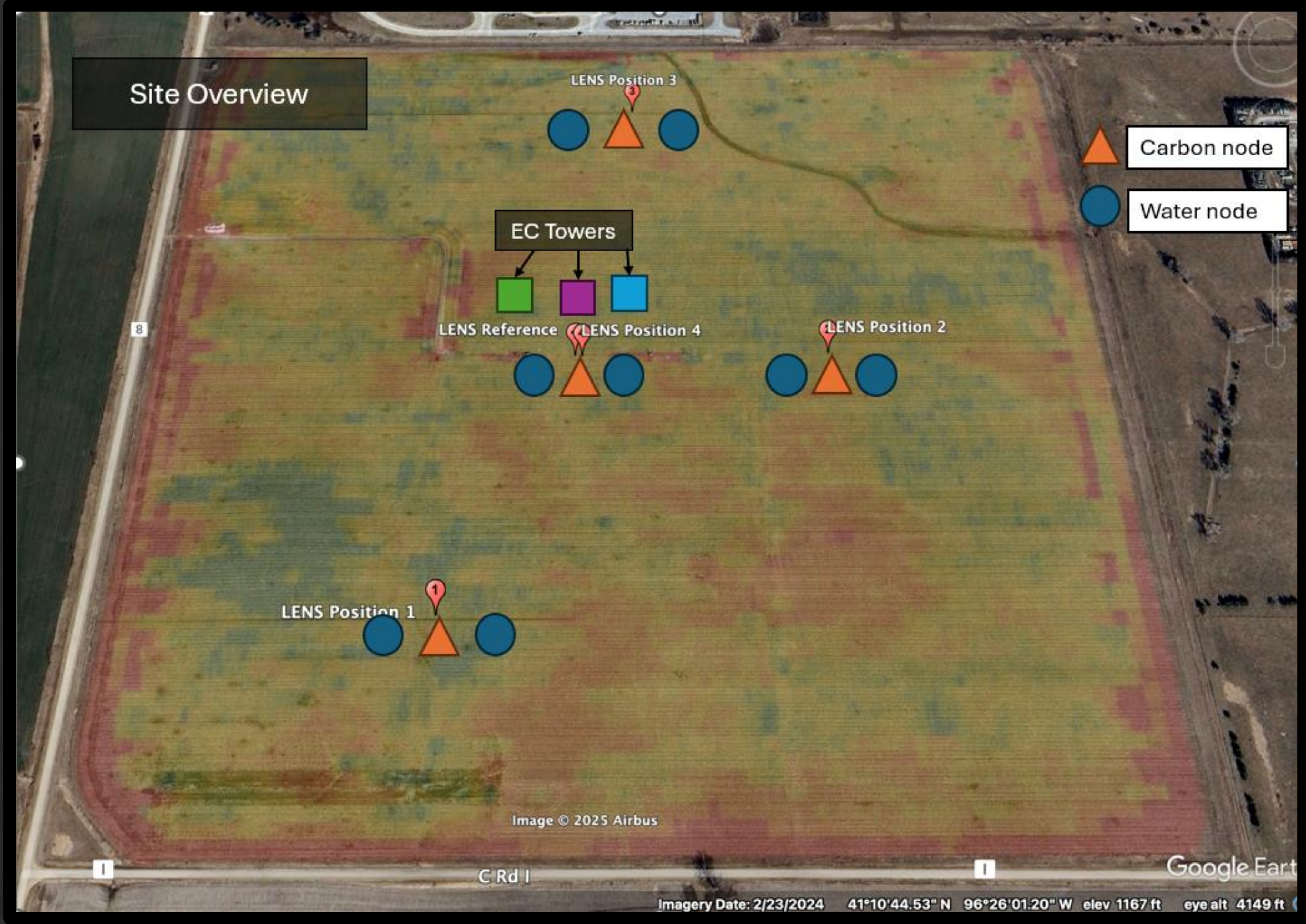
Figure 1: Aerial view of the study field showing the spatial arrangement of carbon nodes (triangles), water nodes (circles), and eddy covariance (EC) towers across four LENS positions. Sensors were deployed to capture fine-scale spatial variability in CO 2 fluxes and evapotranspiration within the EC tower footprint.
