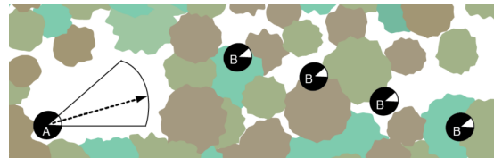
Figure 2. Use a narrow view cap when sampling irregular woodland canopies. Take an Above (A) reading in a clearing and Below (B) readings across a representative transect.
