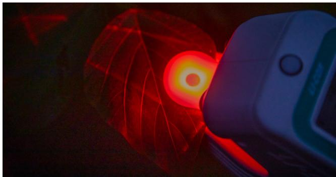
For dark-adapted leaves, the LI-600 measures maximum quantum yield ( $F_v/F_m$ ), or the maximum proportion of absorbed light that can be used to drive electron transport.  $F_v$  is variable fluorescence yield in a dark-adapted leaf;  $F_m$  is maximum fluorescence yield in a dark-adapted leaf;  $F_o$  is minimum fluorescence yield in a dark-adapted leaf.
