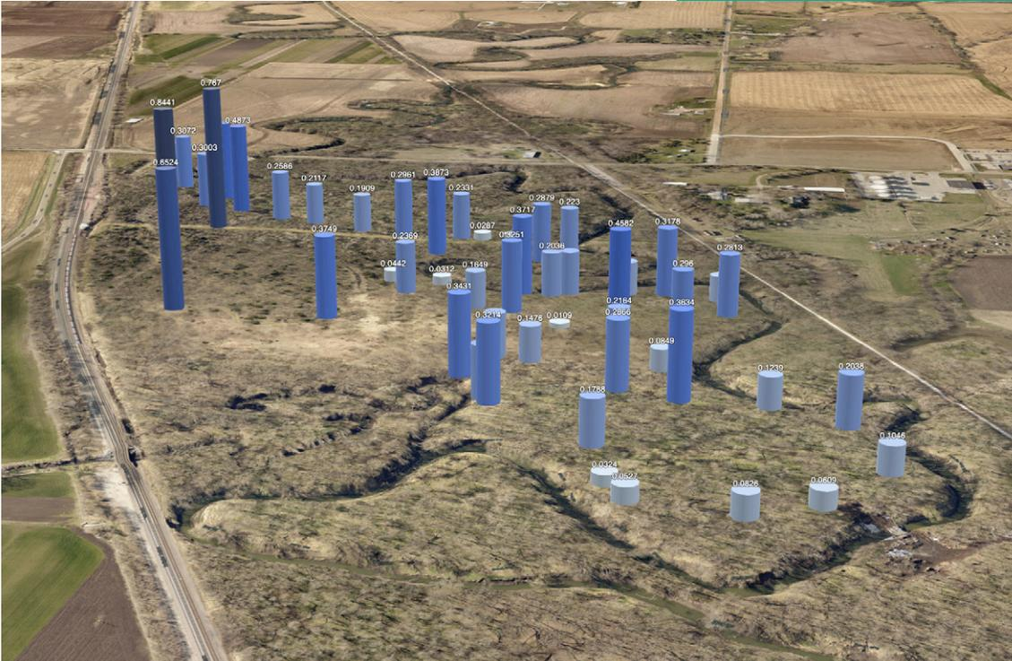
**Figure 1.** Stomatal conductance ( $g_{sw}$ ) measured with a GPS-enabled LI-600. Georeferenced measurements from the LI-600 are easily viewed in mapping applications including Google Earth™ and Esri® ArcGIS®.
