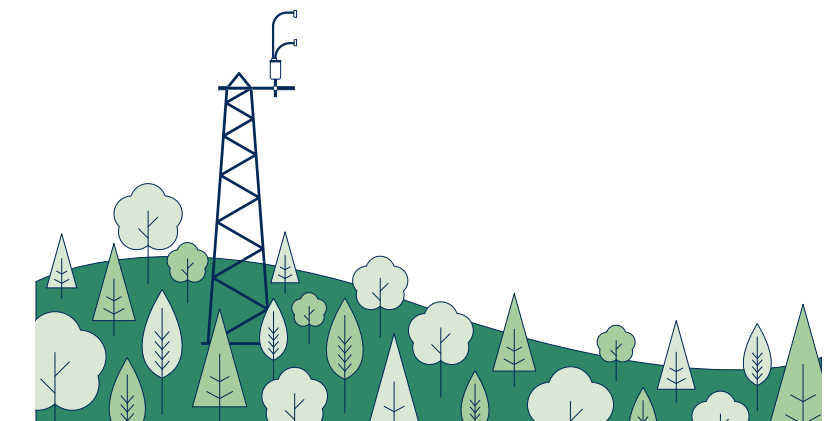
Figure 5. The LI-710 should be 2 to 4 meters above the top of orchards, woodland, and forest canopies.
