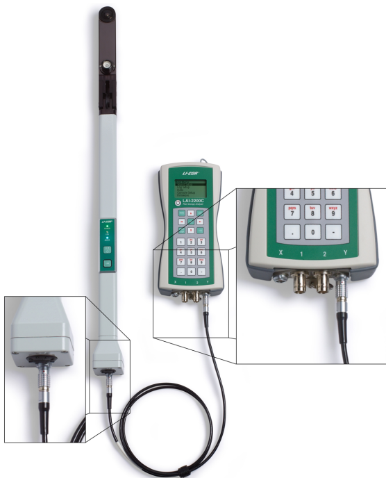
Figure 2-1. The cable connects to the wand and console. The red dot on the cable connector should be oriented to the keypad. To remove the cable, grasp the connector and pull.
