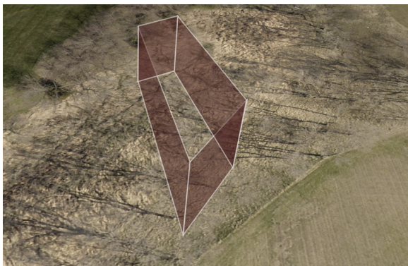
Figure 3-2. Plot marked by GPS Tagging. At each corner of the plot, the "1" key was pressed while a file was open to log a GPS record. A different numeric key could be used to mark other plots in the same file.
