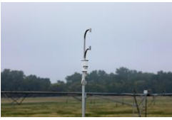
Figures 1,2,3: LI-710 and conceptual representation of the eddy covariance method to quantify fluxes over a landscape.
