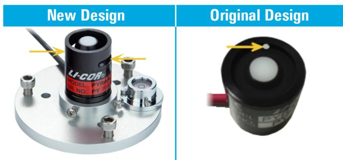
New sensors provide improved water shedding and drainage than the original design.
